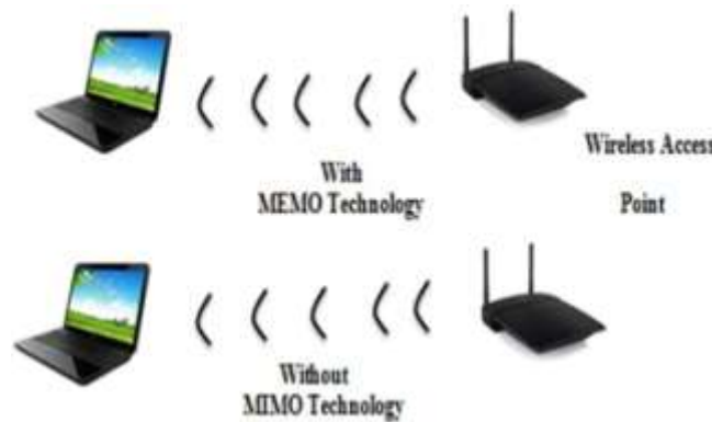
Figure 1 MIMO Technology uses multiple radios to transfer more data at the same time [4]
